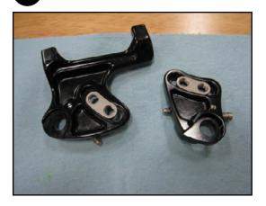
Check motion of adjuster screw. Screw should turn easily, and there should be a firm, audible "click" every ¼ turn
