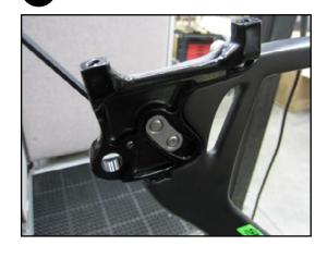
When adjusting chain tension/wheel position, it is recommended to start in the full forward position, and count clicks out as a reference between DS and NDS adjustment.
