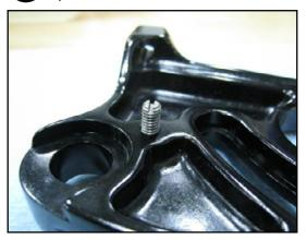
Apply ONE drop of blue Loctite 242 or equivalent
