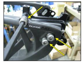
Adjust dropout until bottomed out in the forward position
