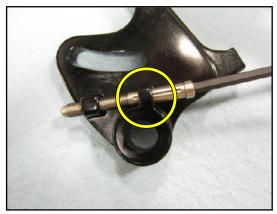
Install detent screw about two threads in by hand
