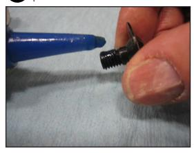
Apply grease to the outside of the shock pin
