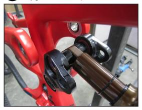
Install shock pin bolt on DS of upper link and torque to 13Nm
