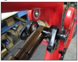
Apply Loctite 243 or equivalent to shock pin bolt threads
