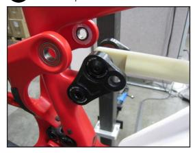
Use an M8 hex wrench to remove rear traingle bolts from the upper link
