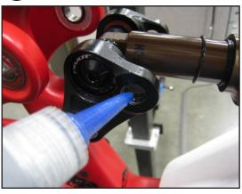
Apply grease to the threads of the front shock bolt
