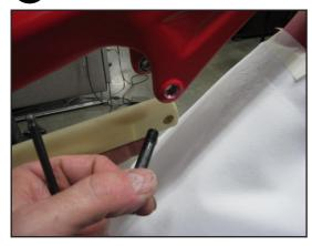
Remove the shock pin, bolt, spacers, and shock using an M5 and M8 hex wrench
