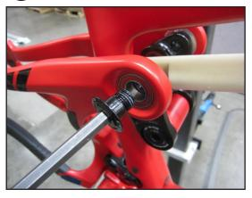
Use an M5 hex wrench to remove the front shock bolt
