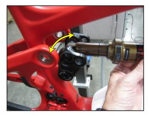
Use a toothpick to spread the Loctite to coat the threads
