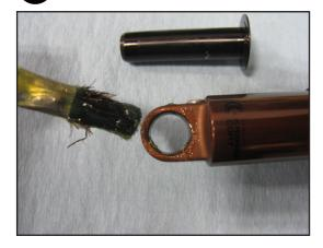
Insert the pin in the NDS bearing and pass through the NDS spacer and shock
