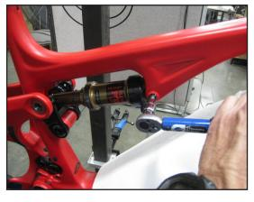
Apply Loctite 243 or equivalent to the upper link (both sides)
