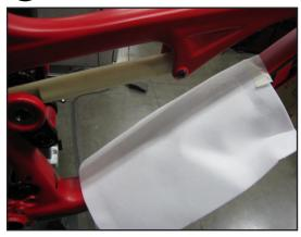
Roll the upper link forward to access the rear shock pin and bolt
