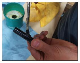
Install the pin with the DS spacer. Clean any grease from the pin threads.
